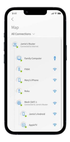
From the dashboard you can select "My Network". This will show any GigaCenter, GigaSpire BLAST, or GigaMesh units connected in your network. Next tap into your Wi-Fi network from the Networks tab. From here, tap into the "Map" section to view devices connected to your system. You can tap on the Mesh icon to get performance information and devices connected at that Mesh unit.
